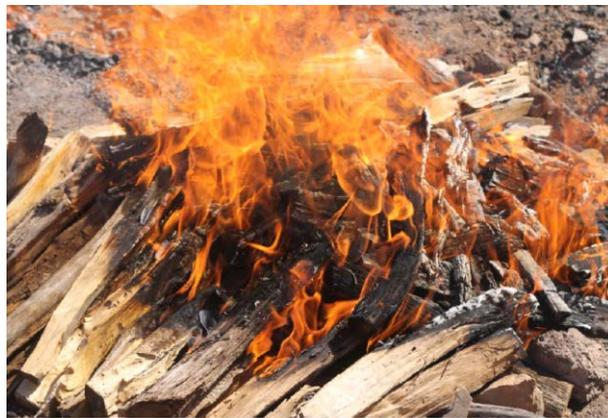
**Figure 10.** The secondary fire is shown here under way. Small diameter fuel means the crib is tight, and this keeps the “fire box” below from getting too much O<sub>2</sub> “on the way up” and oxidizing (burning off) the paint. Combustion is not an issue with dry small diameter fuel which burns more easily for a given amount of O<sub>2</sub> than large fuel due to standard surface/volume scaling (Photo by the author: 2014, Apache Junction, AZ).
