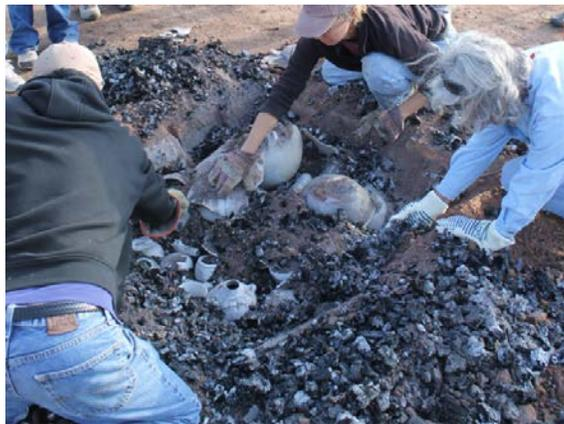
**Figure 4.** After 18-24 hours for cool down, the kiln is excavated to remove the layer of dirt and copious quantities of charcoal left by the smothering. (Photo by author: 2011 Leupp Kiln Conference, Pecos, NM)
