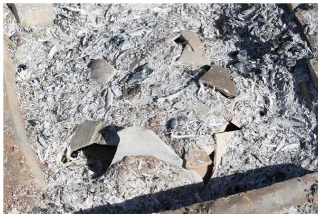
**Figure 11.** As the crib collapses the ash forms a natural blanket that keeps the organic paint from oxidation. While some ash is inevitably blown away as the kiln cools, if the kiln has been built and situated properly it occurs so slowly that by the time the pots are exposed to substantial O<sub>2</sub> they are cool enough so the black is stable. Here, cover sherds are starting to show through the ash. (Photo by the author: 2014, Apache Junction, AZ).
