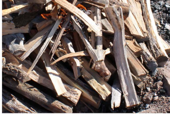
Figure 9. A crib is built beginning with “spanners” going the long length of the kiln of about 2”-2 1/2” in diameter (not shown) and “rafters” 1”-2” in diameter (shown) are placed across the spanners. Smaller pieces (also shown) are used on top to start the fire. (Photo by the author: 2014, Apache Junction, AZ).
