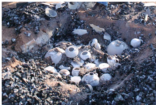
Figure 19. A kiln fired with the SP after firing showing the large quantities of charcoal that result from a single firing both in the kiln and in piled around it. See also Figs. 4, and 5. (Photo by author: 2011 Leupp Kiln Conference, Pecos, NM)
