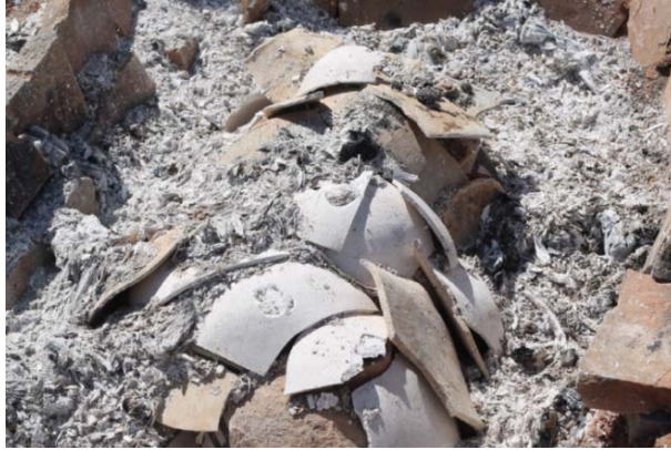
Figure 12. Shortly before being cool enough to open a good portion of the cover sherds have had the ash blown off them. At this point O 2 at or near PAL (present atmospheric levels) is reaching the pots, but they are cool enough so the black is not altered. Whereas a dirt-covered firing takes 18-24 hours to cool down, a kiln fired with the NSP is ready to open the same day in 5 or 6 hours. (Photo by the author: 2014, Apache Junction, AZ)
