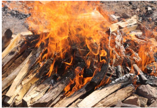
Figure 10. The secondary fire is shown here under way. Small diameter fuel means the crib is tight, and this keeps the “fire box” below from getting too much O 2 “on the way up” and oxidizing (burning off) the paint. Combustion is not an issue with dry small diameter fuel which burns more easily for a given amount of O 2 than large fuel due to standard surface/volume scaling (Photo by the author: 2014, Apache Junction, AZ).
